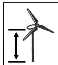
**Wind generator.** The blades and associated mechanical and electrical conversion components mounted on top of the tower whose purpose is to convert kinetic energy of the wind into rotational energy used to generate electricity.
